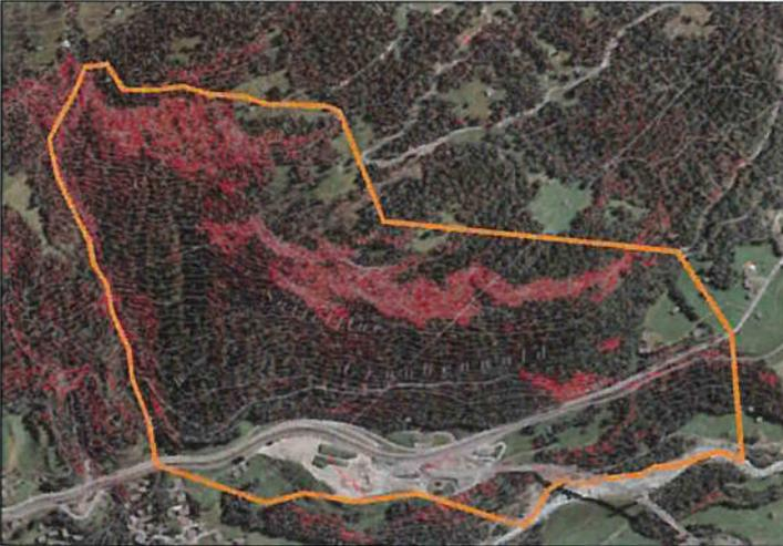
Aerial photograph of a forested area. A large, irregularly shaped region is highlighted in red, indicating potential landslide sites with slopes greater than 45 degrees. The red shading covers a significant portion of the forested hillside. The surrounding area shows a mix of green forest and open fields. A road or path is visible at the bottom of the image.
